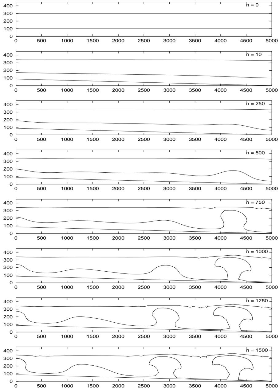
Figure 4: Salt migration initiated by a gradual lift of base rock to an angle of one degree at the initial 10 time steps on the left side. The figures show the growth sequence from right to the left for the appearance of salt structures.
